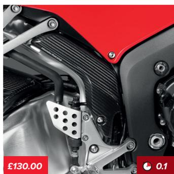
**CARBON-FIBRE EXHAUST GUARD**
