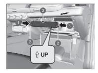
**4.** Push in the tabs on the corners of the filter case cover, and remove it.
