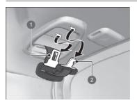
**1.** Pull out the seat belt's small latch plate and the latch plate from each holding slot in the ceiling.
