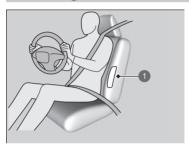
The side airbags are housed in the outside edge of the driver's, passenger's and rear outboard seat-backs.
