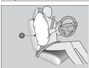
When the sensors detect a moderate-tosevere side impact, the control unit signals the centre airbag to deploy.
