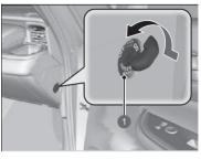
Passenger Front Airbag ON/ OFF Switch
