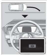
The front camera located at the top of the windscreen monitors left and right lane markings in white or yellow, the outer edge of the pavement (bordered by grass or gravel) or a detected oncoming vehicles.
