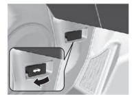
Locate the bonnet latch lever, push it to the side, and then raise the bonnet. Once you have raised the bonnet slightly, you can release the lever.
