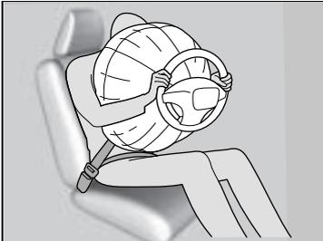
While your seat belt restrains your torso, the front airbag provides supplemental protection for your head and chest. The front airbags deflate immediately so that they won't interfere with the driver's visibility or the ability to steer or operate other controls.
