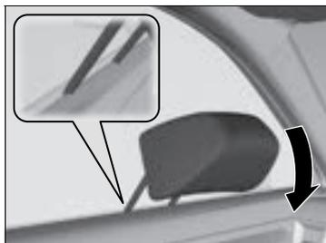
2. Insert the head restraint legs into the lower centre of the front door window.
