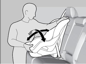
7. Make sure the child restraint system is firmly secured by rocking it forward and back, and side to side; little movement should be felt.
