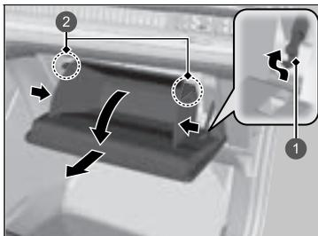
2. Push the stopper on the passenger's side of the glove box to detach it from the glove box.
