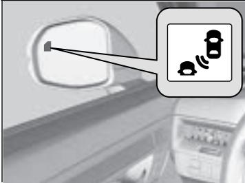
When the following conditions are met and you are making a lane change where there is a risk of collision with a vehicle in the adjacent lane approaching from behind, the Lane Change Collision Mitigation indicator blinks, audible and visual alerts are given, and the system assists steering for collision avoidance.
