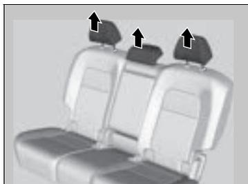
1. Remove the rear seat head restraint.
