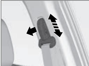
1. Move the anchorage up and down while pulling the shoulder anchorage outward.
