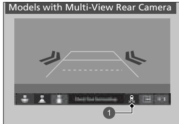
The system can be turned on and off on the audio/information screen by pressing the Cross Traffic Monitor icon.
