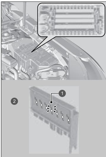
4. Check the combined fuses in the engine compartment fuse box.
