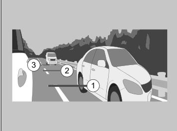
Three lines that appear on the screen can give an idea of how far the vehicles or objects on the screen are from your vehicle, respectively. If an object is near line ① (in red), it indicates that it is close to your vehicle whereas an object near line ③ is farther away.
