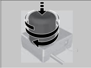
5. Screw the sealed bottle onto the air compressor.
