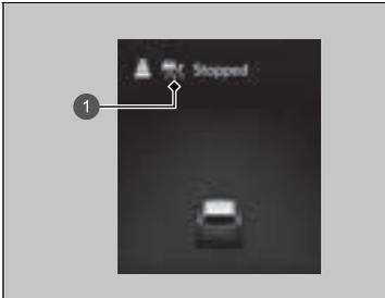
If no vehicle is ahead of you before you resume driving, depress the accelerator pedal and ACC with Low Speed Follow will operate again within the prior set speed.
