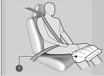
① Deployed Passenger's Knee Airbag
