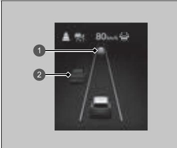
When a vehicle whose speed is slower than your set speed comes in or cuts in front of you and is detected by the radar and the camera, your vehicle starts to slow down.
