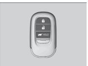
Use the keys to turn on and off the power system, and lock and unlock all the doors, tailgate, and fuel fill door.
