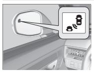
When the following conditions are met and you are making a lane change where there is a risk of collision with a vehicle in the adjacent lane approaching from behind, the Lane Change Collision Mitigation indicator blinks, audible and visual alerts are given, and the system assists steering for collision avoidance.
