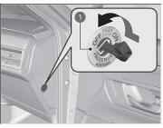
Passenger Front Airbag ON/ OFF Switch
