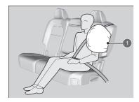
Deployed Side Airbag
