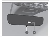
automatic dimming rearview mirror reduces the glare from headlights behind you. Press the AUTO button to turn this function on and off. When activated, the AUTO indicator comes on.
