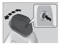
The front head restraint tilt can be adjusted according to you and a front passenger's head positions.
