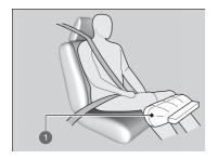
Deployed Passenger's Knee Airbag
