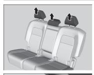
**1.** Remove the rear seat head restraint. **▶ Head Restraints** P. 261
