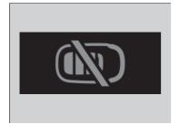
When the power mode is set to any mode other than OFF and you remove the keyless remote from the vehicle and shut the door, an alarm will sound. If the alarm continues to sound, place the keyless remote in another location.
