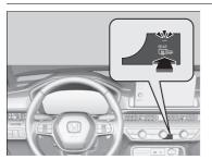
Press the rear demister and heated door mirror button to demist the rear window and mirrors when the power mode is in ON.
