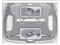
The tie-down anchorages on the luggage area floor can be used to install a net for securing items.
