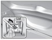
2. Wrap a cloth around the flat-tip screwdriver. Put it into the lid as shown in the image, and open the lid.
