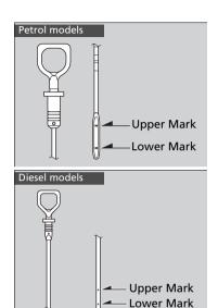
**4.** Remove the dipstick again, and check the level. It should be between the upper and lower marks. Add oil if necessary.
