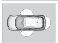
When you carry the keyless remote, you can lock/unlock the doors and tailgate. You can lock/unlock the doors and the tailgate within a radius of about 80 cm (32 inches) of the outside door handle. You can open the tailgate within about 80 cm (32 inches) radius from the tailgate release button.
