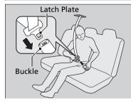
**3.** Insert the latch plate into the buckle. Properly fasten the seat belt the same way you fasten the lap/shoulder seat belt.
