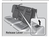
Pull the lever on the right to change the angle of the right half of the seat-back, and left for the left half.
