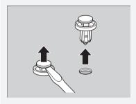
Insert the clip with the centre pin raised, and push until it is flat.
