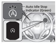
The engine then restarts once the vehicle is about to move again when you depress the clutch pedal, and the indicator (green) goes off.
