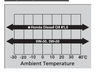
Use a commercial engine oil of suitable viscosity for the ambient temperature as shown.
