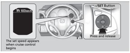
Take your foot off the accelerator pedal and press the **–/SET** button when you reach the desired speed.
