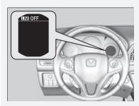
If there is a problem with the system when you are using the adjustable speed limiter, the beeper sounds and **OFF** comes on. The adjustable speed limiter will be turned off.
