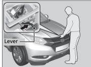
**3.** Push the bonnet latch lever in the centre of the bonnet to release the lock mechanism, and open the bonnet.
