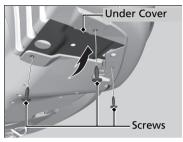
**1.** Remove the screws using a Phillips-head screwdriver, then push up the under cover.
