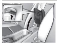
Pull the handle to open the console compartment.
