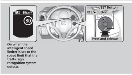
• The moment you release the **-/SET** button or **RES/+** button, the intelligent speed limiter is set to the speed limit that the traffic sign recognition system detects. The speed limit is displayed.
