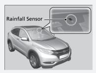
Do not put the wiper lever in **AUTO** when cleaning the windscreen or driving through a car wash. If the wiper lever is in **AUTO**, and the ignition switch is in ON  $\boxed{\text{II}}^{*_1}$ , the rainfall sensor may respond to your hand or car wash liquids, and the wipers may operate automatically.
