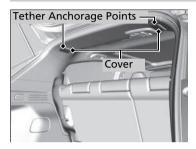
Two tether anchorage points are provided on the ceiling for rear outer seating positions. A child restraint system that is installed with a seat belt and comes with a tether can use the tether for additional security.
