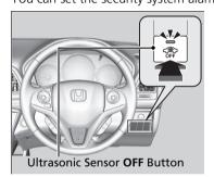
To turn off the ultrasonic sensor system, press the ultrasonic sensor **OFF** button after you remove the key from the ignition switch, or with the key in the ACCESSORY  $\square$  or LOCK  $\boxed{0}^{*1}$ .
