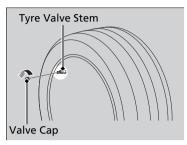
**1.** Remove the valve cap from the tyre valve stem.
