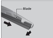
**3.** Slide the wiper blade out from the end with the indent.
