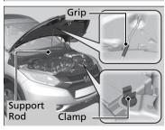
**4.** Remove the support rod from the clamp using the grip. Mount the support rod in the bonnet.
