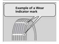
The groove where the wear indicator is located is 1.6 mm (1/16 inch) shallower than elsewhere on the tyre. If the tread has worn so that the indicator is exposed, replace the tyre. Worn out tyres have poor traction on wet roads.
