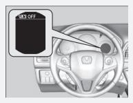
If there is a problem with the system or traffic sign recognition system when you are using the intelligent speed limiter, the beeper sounds and **OFF** comes on. The intelligent speed limiter will be turned off.
