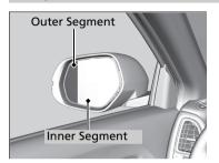
The driver's side door mirror has outer and inner segments.
