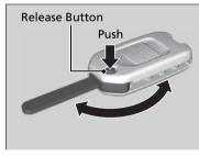
The key folds up inside the remote transmitter.
