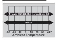
Use a commercial engine oil of suitable viscosity for the ambient temperature as shown
