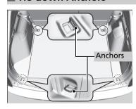
The tie-down anchors on the luggage area floor can be used to install a net for securing items.
