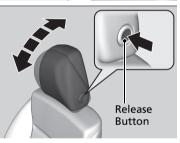
**To tilt the head restraint forward:** Push the back of it forward.
