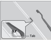
**2.** Press and hold the tab, then slide the blade from the wiper arm.
