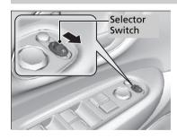
If activated, passenger side door mirror automatically tilts downward when you put the shift lever in  $\boxed{R}$ ; this improves close-in visibility on the passenger side of the vehicle when reversing. The mirror automatically returns to its original position when you shift out of  $\boxed{R}$ .
