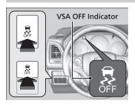
This button is on the driver side control panel. To partically turn the VSA features on and off, press and hold it until you hear a beep.
