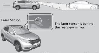
The system activates when the speed difference between your vehicle and a vehicle detected in front of you is about 5 km/h (3 mph) to 32 km/h (20 mph) with a high chance of collision.
