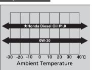
Use a commercial engine oil of suitable viscosity for the ambient temperature as shown.
