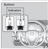
Press the Lane Departure Warning button to turn the system on and off.
