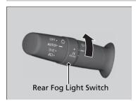
■ To turn the rear fog light on Rotate the switch to O‡. The O‡ indicator comes on.
