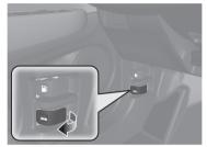
2 Locate the bonnet latch lever, push the lever and lift up the bonnet.
