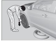
**7.** Loosen each wheel nut about one turn using the wheel nut wrench.
