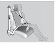
The tensioners automatically tighten the front and rear outer seat belts during a moderate-to-severe frontal collision, sometimes even if the collision is not severe enough to inflate the front airbags.
