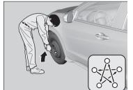
**5.** Lower the vehicle and remove the jack. Tighten the wheel nuts in the order indicated in the image. Go around, tightening the nuts, two to three times in this order.
