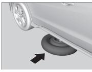
**6.** Place the spare tyre (wheel side up) under the vehicle body, near the tyre that needs to be replaced.
