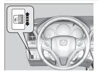
You can adjust the vertical angle of the low beam headlights when the ignition switch is in ON  $\boxed{II}^{*1}$ .
