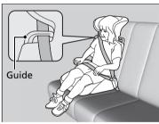
A back-rest is available for a specific booster seat. Install the back-rest to the booster seat and adjust it to the vehicle seat according to the booster seat manufacturer's instructions. Make sure the seat belt is properly routed through the guide at the shoulder of the back-rest and the belt does not touch and cross the child's neck.
