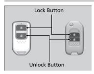
**To open:** Press the unlock button twice within 10 seconds and hold it down for the second time.
