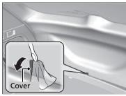
**1.** Wrap a cloth around the flat-tip screwdriver. Put it into the cover as shown in the image, and open it.
