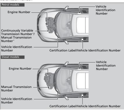
■Vehicle Identification Number (VIN), Engine Number and Transmission Number
