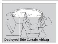
The side curtain airbag is designed to deploy in a moderate-to-severe side impact.
