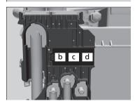
Pull up the cover on the  $\oplus$  terminal, then remove it while pulling out the tab as shown.
