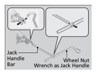
**3.** Raise the vehicle, using the jack handle bar and the jack handle, until the tyre is off the ground.
