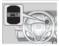
The beeper sounds, and a find blinks on the multi-information display, and hard braking is applied when a possible collision becomes likely unavoidable.
