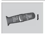
When you push the lever down to **AUTO**, the windscreen wipers sweep once, and go into the automatic mode.
