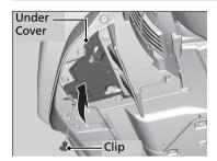
**1.** Remove the clip using a flat-tip screwdriver, and push up the under cover.
