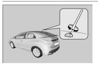
Your vehicle is equipped with a removable antenna at the rear of the roof.
