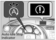
The engine then restarts once the vehicle is about to move again when you depress the clutch pedal, and the indicator goes off. A message associated with Auto Idle Stop appears on the i-multi-information display.
