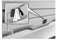
**1.** Use a flat-tip screwdriver and remove the cover on the back of the tailgate.
