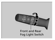
■ To turn the front fog lights on Rotate the switch up from the OFF position to the 釣 position. The 鉤 indicator comes on.
