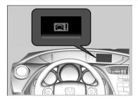
The beeper sounds, and a CTBA warning blinks on the i-multi-information display, and hard braking is applied when a possible collision becomes likely unavoidable. This automatic braking with the system activated is cancelled after the vehicle comes to a complete stop.
