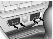
The indicator for your setting comes on while the seat heater is in use. Briefly press the button on the opposite side to turn the heater off. The indicator goes off. While in **HI**, the heater cycles on and off. When a comfortable temperature is reached, select **LO** to keep the seat warm.
