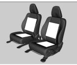
The ignition switch must be in ON  $\boxed{II}^{*1}$  to use the seat heaters. The **HI** setting heats the seats faster than the **LO** setting.
