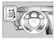
You can adjust the vertical angle of the low beam headlights when the ignition switch is in ON  $[II]^{*1}$ .
