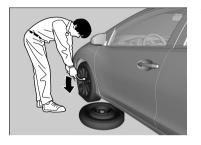
**11.**Loosen each wheel nut about one turn using the wheel nut wrench.
