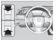
Turn the headlights on and press the headlight washer button to operate. The headlight washers also operate when you turn the windscreen washers for the first time after the ignition switch is in ON  $[II]^{*1}$ .
