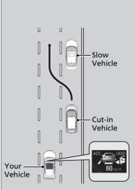
The radar sensor in the lower bumper detects vehicles ahead of you including those in the adjacent lane, and the camera behind the rearview mirror detects the lane markings.
