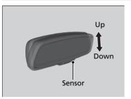
When you are driving after dark, the automatic dimming rearview mirror reduces the glare from headlights behind you, based on inputs from the mirror sensor. This feature is always active. ➢Automatic Dimming Rearview Mirror\*
