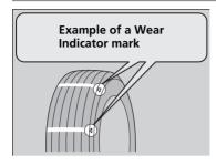
The groove where the wear indicator is located is 1.6 mm (1/16 inch) shallower than elsewhere on the tyre. If the tread has worn so that the indicator is exposed, replace the tyre. **Worn out tyres have poor traction on wet roads.**
