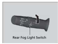
■ To turn the rear fog light on Rotate the switch to ()‡. The ()‡ indicator comes on.
