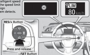
• The moment you release the –/SET button or RES/+ button, the intelligent speed limiter is set to the speed limit that the traffic sign recognition system detects. The speed limit is displayed.
