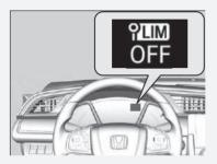
If there is a problem with the system or traffic sign recognition system when you are using the intelligent speed limiter, the beeper sounds and **OFF** comes on. The intelligent speed limiter will be turned off.
