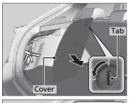
**2.** Turn and pull the tab to open the compartment cover located on the left side of the luggage area.
