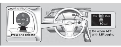
When driving at about 30 km/h (18 mph) or above: Take your foot off the pedal and press the –/SET button when you reach the desired speed. The moment you release the button, the set speed is fixed, and ACC with LSF begins.
