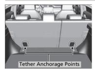
Two tether anchorage points are located behind each rear outer seating positions. If you have a child restraint system that comes with a tether but can be installed with a seat belt, the tether may be used for additional security.
