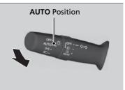
Disable or re-enable the system when the vehicle is parked and the ignition switch is in ON  $\boxed{II}^{*1}$  and the light switch is in the **AUTO** position.
