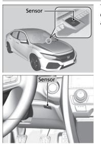
The automatic climate control system is equipped with sensors. Do not cover or spill any liquid on them.
