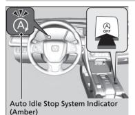
To turn the Auto Idle Stop system off, press this button. The Auto Idle Stop system stops.
