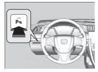
With the ignition switch in ON  $III^{*1}$ , press the parking sensor system button to turn on or off the system. The indicator in the button comes on when the system is on.
