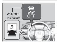
This button is on the driver side control panel. To partially disable VSA functionality/ features, press and hold it until you hear a beep.
