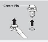
Insert the clip with the centre pin raised, and push until it is flat.
