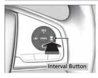
Press the 🖹 (interval) button to change the ACC with LSF following-interval. Each time you press the button, the following-interval (the interval behind a vehicle detected ahead of you) setting cycles through extra long, long, middle, and short following-intervals.
