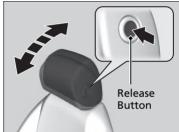
To tilt the head restraint forward: Push the back of it forward. To tilt the head restraint backward: Push it backward while pressing the release button on the side of the head restraint.
