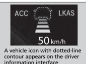
Your vehicle maintains the set speed without having to keep your foot on the brake or accelerator pedal. If there previously was a vehicle detected
