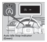
If the driver's door is opened while the indicator (green) is on, a buzzer sounds to notify you that the Auto Idle Stop function is in operation.
