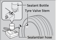
**1.** Remove the valve cap from the tyre valve stem.
