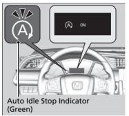
The engine then restarts once the vehicle is about to move again, or depending on environmental and vehicle conditions, and the indicator (green) goes off.
