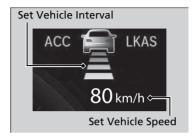
When ACC with LSF starts operating, the vehicle icon, interval bars and set speed appear on the driver information interface.
