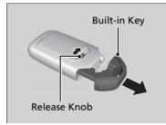
The built-in key can be used to lock/unlock the doors when the keyless remote battery becomes weak and the power door lock/ unlock operation is disabled. To remove the built-in key, slide the release knob and then pull out the key. To reinstall the built-in key, push the built-in key into the keyless remote until it clicks.
