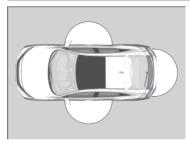
When you carry the keyless remote, you can lock/unlock the doors and hatch. You can lock/unlock the doors and hatch within a radius of about 80 cm (32 inches) of the outside door handle or hatch release button.
