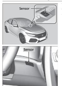
The automatic heating system is equipped with sensors. Do not cover or spill any liquid on them.
