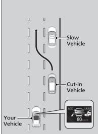
The radar sensor in the lower bumper detects vehicles ahead of you including those in the adjacent lane, and the camera behind the rearview mirror detects the lane markings.
