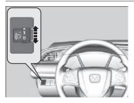
You can adjust the vertical angle of the low beam headlights when the position lights are on.
