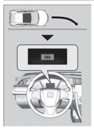
The front camera behind the rearview mirror monitors left and right lane markings (in white or yellow). If your vehicle is getting too close to detected lane markings without a turn signal activated, the system, in addition to a visual alert, applies steering torque and alerts you with rapid vibrations on the steering wheel, to help you remain within the detected lane. Customized Features\* P. 156
