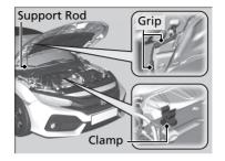
**4.** Remove the support rod from the clamp using the grip. Mount the support rod in the bonnet.
