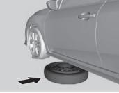
**7.** Place the spare tyre (wheel side up) under the vehicle body, near the tyre that needs to be replaced.
