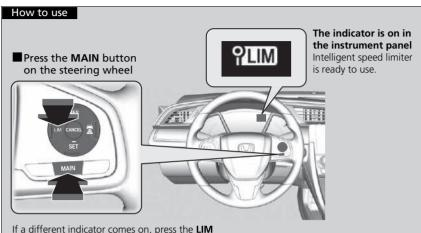
If a different indicator comes on, press the **LIM** button to change it to the intelligent speed limiter.
