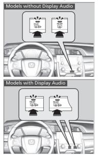
The rear demister and heated door mirrors automatically switch off after 10-30 minutes depending on the outside temperature. However, if the outside temperature is 0°C or below, they do not automatically switch off.
