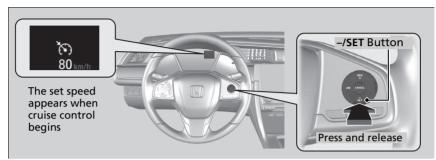
Take your foot off the accelerator pedal and press the **–/SET** button when you reach the desired speed.
