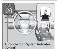
To turn the Auto Idle Stop system off, press this button. The Auto Idle Stop system stops. ► Auto Idle Stop system will stop and the indicator (amber) will come on.
