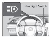
To activate the system, turn the headlight switch to **AUTO** and then set the headlights to low beam. The auto high-beam indicator will come on.
