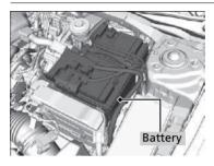
The condition of the battery is monitored by a sensor located on the negative terminal of the battery. If there is a problem with this sensor, the driver information interface will display a warning message. If this happens, have you vehicle inspected by a dealer.
