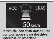
Your vehicle maintains the set speed without having to keep your foot on the brake or accelerator pedal.
