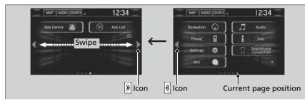
Selecting  $\langle\!\!\langle\!\!\langle$  or  $\rangle\!\!\rangle_{\!\!\!}$ , or swiping the screen left or right changes to the next screen.
