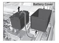
6. Remove the battery cover.7. Take out the battery carefully.
