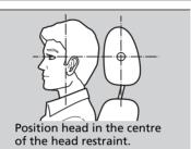
Front head restraints are most effective for protection against whiplash and other rearimpact crash injuries when the centre of the back of the occupant's head rests against the centre of the restraint. The tops of the occupant's ears should be level with the centre height of the restraint.
