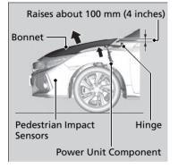
When the pedestrian impact sensors detect a certain amount of impact, the pop-up hood system is activated and the rear of the bonnet will raise.
