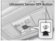
To turn off the ultrasonic sensor system, press the ultrasonic sensor OFF button after you remove the key from the ignition switch, or with the key in the ACCESSORY  $\boxed{1}$  or LOCK  $\boxed{0}^{*1}$ .
