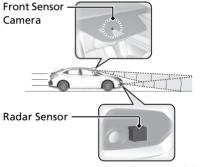
The radar sensor is in the lower bumper.
