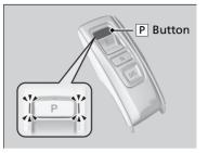
The gear position changes to  $\mathbf{P}$  when you press the  $\mathbf{P}$  button while the vehicle is parked with the power mode in ON. The indicators on the sides of the  $\mathbf{P}$  button come on.
