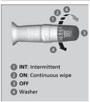
The rear wiper and washer can be used when the ignition switch is in ON  $[II]^{*1}$ .
