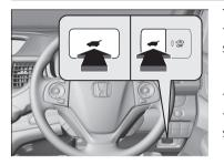
To open: Press and hold the tailgate button in the driver side control panel for about one second.
