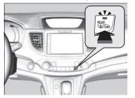
The rear demister and heated door mirrors automatically switch off after 10-30 minutes depending on the outside temperature. However, if the outside temperature is 0°C or below, they do not automatically switch off. ≥Rear Demister/Heated Door Mirror Button
