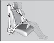
The front seats are equipped with automatic seat belt tensioners to enhance safety.
