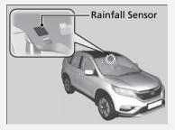
Do not put the wiper lever in **AUTO** when cleaning the windscreen or driving through a car wash. If the wiper lever is in **AUTO**, and the ignition switch is in ON  $\boxed{III}^{*1}$ , the rainfall sensor may respond to your hand or car wash liquids, and the wipers may operate automatically.
