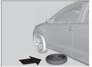
**6.** Place the spare tyre wheel side up under the vehicle body, near the tyre that needs to be replaced.
