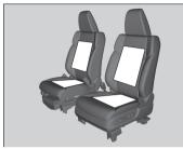
The ignition switch must be in ON  $\boxed{II}^{*1}$  to use the seat heaters. The **HI** setting heats the seats faster than the **LO** setting.
