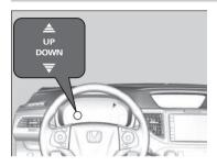
Come on to indicate when a gear change is appropriate to maintain the most fuel efficient driving style.
