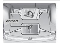
The tie-down anchors on the luggage area floor can be used to install a net for securing items.
