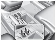
The indicator for your setting comes on while the seat heater is in use. Press the button on the opposite side to turn the heater off. The indicator goes off.
