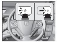
To turn off the ultrasonic sensor system, press the ultrasonic sensor OFF button after you remove the key from the ignition switch, or with the key in the ACCESSORY  $\blacksquare$  or LOCK  $\boxed{0}^{*1}$ .
