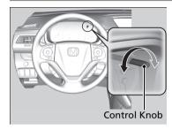
When the position lights are turned on and the ignition switch is in ON III<sup>\*1</sup>, you can use the brightness control knob to adjust instrument panel brightness. **Brighten:** Turn the knob to the right. **Dim:** Turn the knob to the left.
