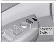
If activated, the passenger side door mirror automatically tilts downward when you change the gear position to  $[\mathbf{R}]$ ; this improves close-in visibility on the passenger side of the vehicle when backing up. The mirror automatically returns to its original position when you change the gear position out of  $[\mathbf{R}]$ .
