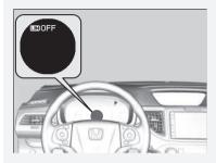
If there is a problem with the system when you are using the adjustable speed limiter, the beeper sounds and the **OFF** comes on. The adjustable speed limiter will be turned off.
