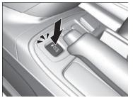
To turn the Auto Idle Stop system off, press this button. The Auto Idle Stop system stops. Auto Idle Stop system will stop and the
