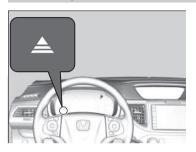
Come on while the vehicle is in the sequential shift mode to indicate when a gear change is appropriate to maintain the most fuel efficient driving style.
