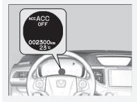
Even though adaptive cruise control has been automatically cancelled, you can still resume the prior set speed. Wait until the condition that caused ACC to cancel improves, then press the **RES/+** button.
