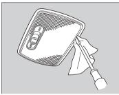
Pry on the edge of the cover using a flattip screwdriver to remove the cover.
