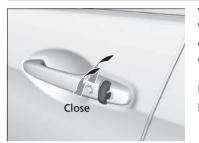
**To close:** Lock the driver's door with the key. Within 10 seconds of returning the key to the central position, turn the key in the lock direction and hold it there.
