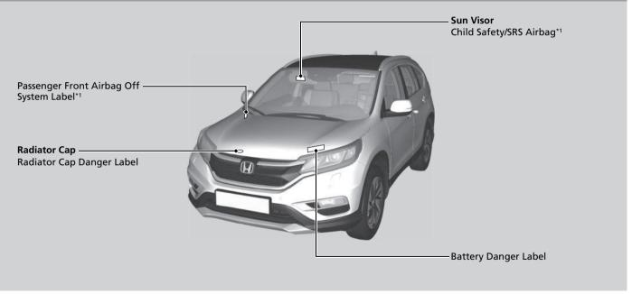
\*1:Left-hand drive models shown. For the right-hand drive models, these labels are located at the symmetrically opposite to the left-hand drive model.
