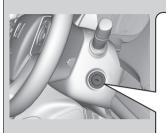
O LOCK: Insert and remove the key in this position.
