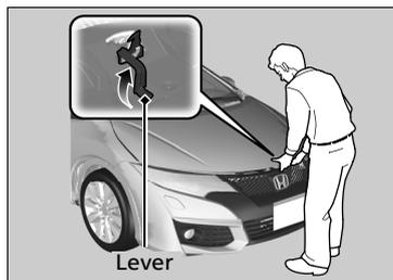
3. Push up the bonnet latch lever in the centre of the bonnet to release the lock mechanism, and open the bonnet.
