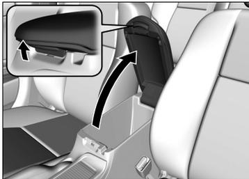
Pull the handle to open the console compartment.
