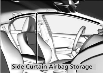
The side curtain airbags are located in the ceiling above the side windows on both sides of the vehicle.
