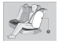
Deployed Side Airbag
