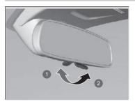
Flip the tab to switch the position. The night position will help to reduce the glare from headlights behind you when driving after dark.
