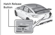
Press the hatch release button to unlock and open the hatch when you carry the keyless remote.
