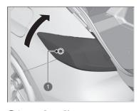
**3.** Grasp underneath the taillight and rotate it upward to release the lower snap pin.
