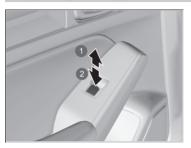
**To open:** Push the switch down. **To close:** Pull the switch up.
