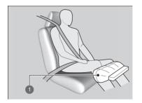
Deployed Passenger's Knee Airbag
