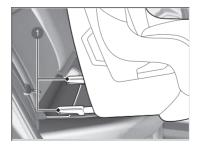
**3.** Place the child restraint system so that the probes are on the cover.
