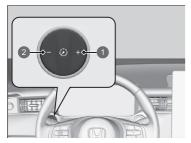
1 + Button 2 - Button The brightness of the gauge is automatically adjusted depending on the ambient brightness.
