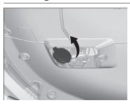
Check the amount of window washer fluid by looking at the reservoir.
