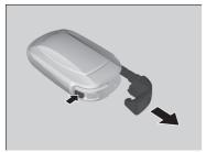
Battery type: Manganese dioxide Lithium battery CR2032
