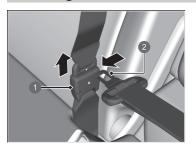
latch plate into the slot on the side of the anchorage buckle.
