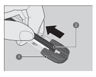
**3.** Pull the end of the wiper blade in the direction of the arrow in the image until it is out of the holder's end cap.
