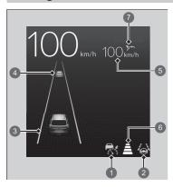
You can see the current status of Adaptive Cruise Control (ACC) with Low Speed Follow, Lane Keeping Assist System (LKAS) and Traffic Jam Assist.
