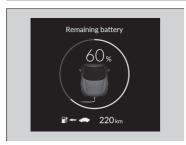
Displays the current status of the High Voltage battery.
