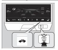
Pressing the (windscreen demister) button turns the air conditioning system on and automatically switches the system to fresh air mode.
