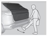
Use a forward and back kicking motion for about 1 second under the centre of the rear bumper to open or close the power tailgate while carrying the keyless remote.
