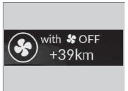
You can increase the driving range by turning off the climate control system. The distance displayed under **with (S) OFF** is the additional estimated distance that the vehicle can drive if the climate control system is turned off.
