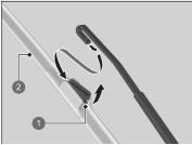
**2.** Press up on and hold the tab, then slide the holder off the wiper arm.
