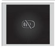
When the power mode is set to any mode other than OFF and you remove the keyless remote from the vehicle and shut the door, an alarm will sound. If the alarm continues to sound, place the keyless remote in another location.
