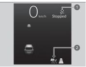
Your vehicle also stops, automatically. The **Stopped** message appears on the gauge. When the vehicle ahead of you starts again, if you press the **RES/+** or **SET/-** button, or depress the accelerator pedal, ACC with Low Speed Follow operates again within the previously set speed.
