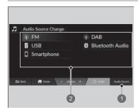
Select **Audio Source** on the middle screen, then select an icon on the source list to switch the audio source.
