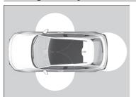
When you carry the keyless remote, you can lock/unlock the doors and tailgate. You can lock/unlock the doors and tailgate within a radius of about 80 cm (32 inches) from the outside door handle or tailgate outer handle.
