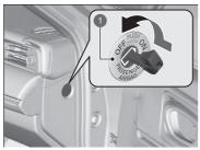
Passenger Front Airbag ON/ OFF Switch
