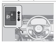
You can adjust the vertical angle of the low beam headlights when the power mode is in ACCESSORY or ON.
