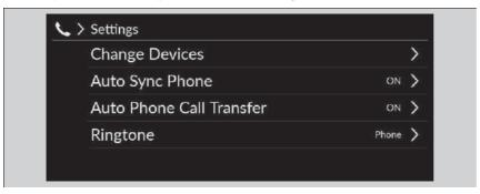
**Change Devices**: Pair a new phone to the system and connect, disconnect, or delete a paired device.
