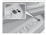
If activated, the passenger side door mirror automatically tilts downward when you put the transmission into  $\boxed{\mathbf{R}}$ : this improves close-in visibility on the passenger side of the vehicle when backing up. The mirror automatically returns to its original position when you take the transmission out of  $\boxed{\mathbf{R}}$ .
