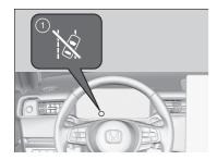
Road Departure Mitigation System Steering Assist Auto OFF indicator If the system operates several times without detecting driver response, the system beeps to alert you. After that, the Road Departure Mitigation System Steering Assist Auto OFF indicator comes on, the Road Departure Mitigation steering assist is temporarily stopped, and the system will only alert you with the warning sound.
