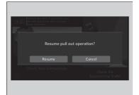
When assistance is able to be resumed, **Resume parking operation?/Resume pull out operation?** will be displayed on the screen. While the brake pedal is depressed, touch the **Resume** icon on the screen and assistance will continue. Release the brake pedal.
