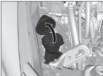
Check the amount of window washer fluid by looking at the reservoir.
