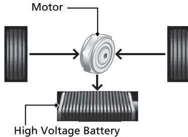
When decelerating without the accelerator being depressed or the brake pedal being applied, or while driving downhill, the electric motor acts as a generator that recovers a portion of the electrical energy that was used to accelerate the vehicle. This regenerative braking slows the vehicle in a manner similar to engine braking in a petrol-powered vehicle. This function is enhanced when the shift lever is moved to **B**.
