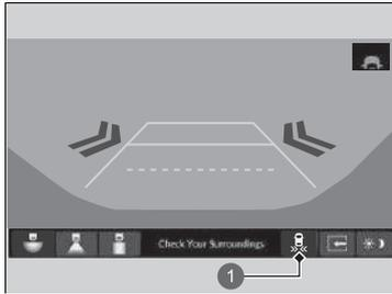
Tap to turn the system on and off. The indicator comes on with the system on. You can also switch the system on and off from the customized feature on the audio/information screen.
