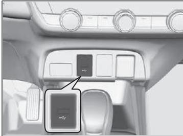
The USB port (1.0A) is for playing audio files on a USB flash drive, connecting a mobile phone, and charging devices.
