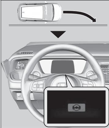
The front camera located at the top of the windshield monitors left and right lane markings in white or yellow, the outer edge of the pavement (bordered by grass or gravel) or a detected oncoming vehicles.
