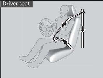
The front seats and the outer rear seats are equipped with automatic seat belt tensioners to enhance safety.
