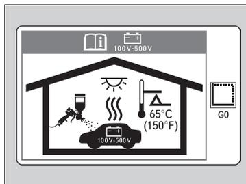
High temperature may damage the high-voltage battery used to power the electric motor.
