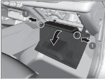
2. Disengage the two tabs by pushing on each side panel.
