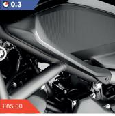
Leg Deflector Kit 08R70-MGS-D10 A set of left and right polyurethane deflectors that fit to the upper fairing and extend the amount of wind protection around the legs for both rider and pillion.
