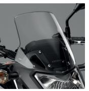
Fly Screen A polycarbonate Fly Screen that provides improved rider comfort by reducing wind blasts on the chest at higher speeds. It is 50mm higher and 40mm wider than the standard version.
