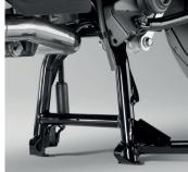
Main Stand (Touring Pack only) A necessity for more secure parking on variable ground surfaces, a Main Stand also eases cleaning and rear wheel maintenance.
