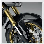
Carbon-Fibre Front Mudguard
