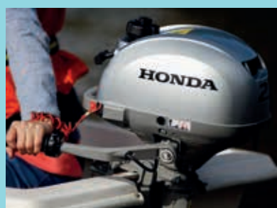
The BF2.3 offers 360° steering for simplified manoeuvrability.
