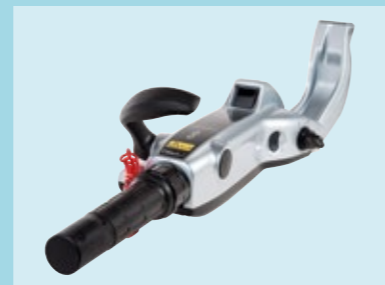
Available as an option, the multi-function tiller handle for BFP60/BF60 incorporates all that you need: power trim-tilt switch, reversible shift lever, handle height adjustment and an engine alert panel.
